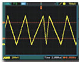
Slope Trigger Triggers on the signals rise time or fall time is user defined
